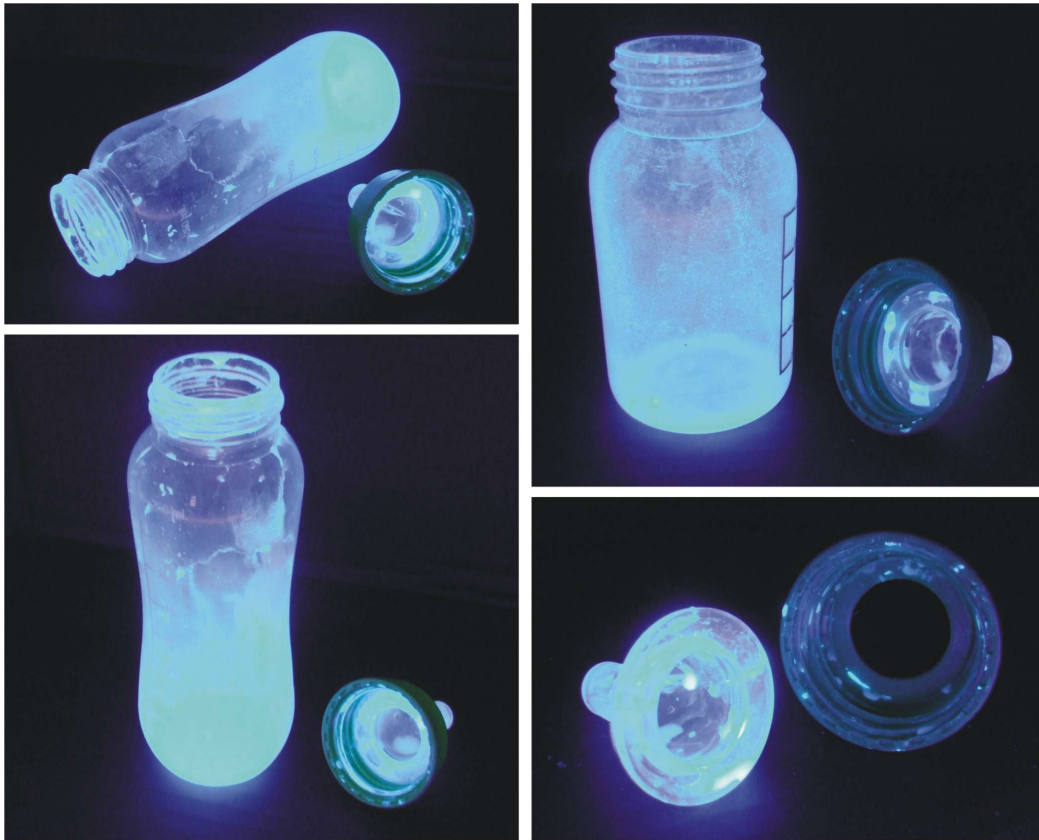
Figure 1 A: Baby bottles into which full cream milk containing 'Glitter Potion' was added, allowed to dry and then photographed under UVA light.
