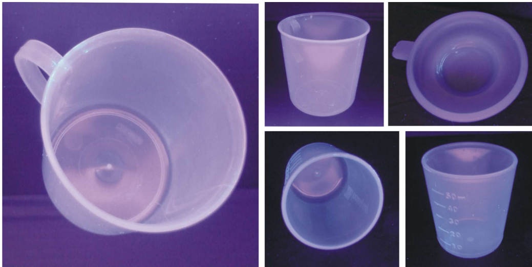
Figure 2 B: Sinapi Feeding Cups into which full cream milk containing 'Glitter Potion' was added, allowed to dry, washed with cold water by hand and then photographed under UVA light.
